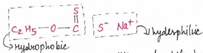
Sulphide ore is absorbed on hydrophilic end while hydrophobic end will act as water repellent which distinguish froth from water.
