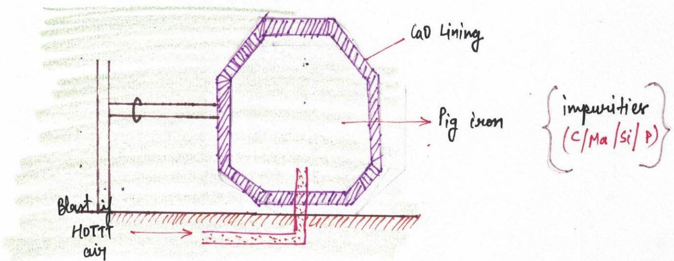
Bessemerisation = (CaO Lining) Puddling ( $\text{Fe}_2\text{O}_3$  lining)
